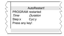
When any key is pressed, the display jumps back to the program view. If the program is to be cancelled, press the (s) key and confirm by
